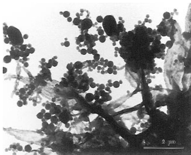
Figure 4. Transmission electron micrograph of "single crystals" of syndiotactic PHB, grown in 5:1 ethanol/chloroform.
